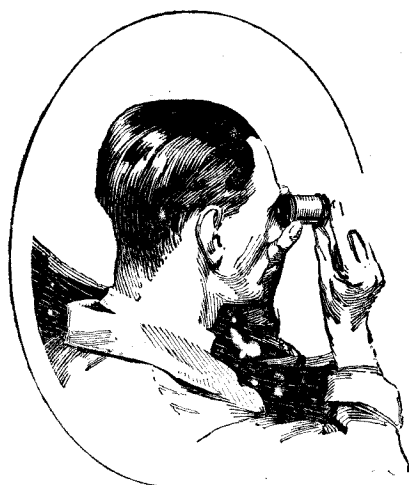
Illustration showing laboratory worker taking a temperature reading by means of the Pyrometer.
